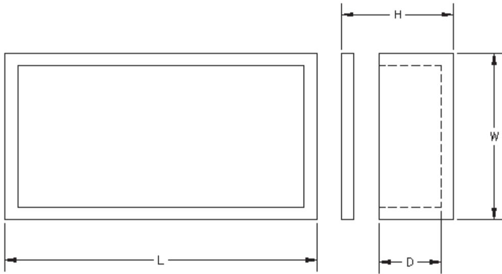
Packages can be fabricated in any dimension within our maximum standard size of  $W = 6''$  and  $L = 12''$ . The height (H) and depth (D) are also selectable and can equal W or 6 inches. This means that almost any configuration from a .250 inch square up to a 6 inch by 12 inch package can be manufactured with very little tooling cost and in quantities starting with one piece.
